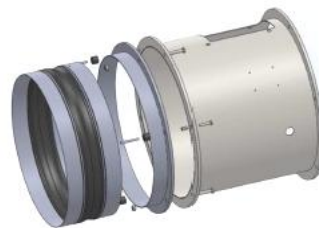
Flexible coupling and mounting pins
